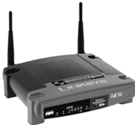
Figure 5-1. Wireless LAN Access Points Connect Wireless LANs to Wired Networks (Photo Courtesy of Linksys)
